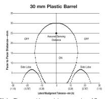
**Note:** There must be a minimum spacing of 7 mm (0.275 in) if actuator and sensor face approaches laterally. This will prevent false triggering due to the side lobe areas.
